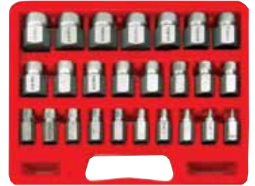
25 PCE MULTI SPLINE EXTRACTOR SET • Remove broken studs, screws, pipes & fittings • Hex head for use with sockets & wrenches • Fine knurled multi spline grips a large cross section compared with std extractors • Tough alloy steel 1/8" (3.2mm) to 7/8" (22.3mm) Part No. RT0305
