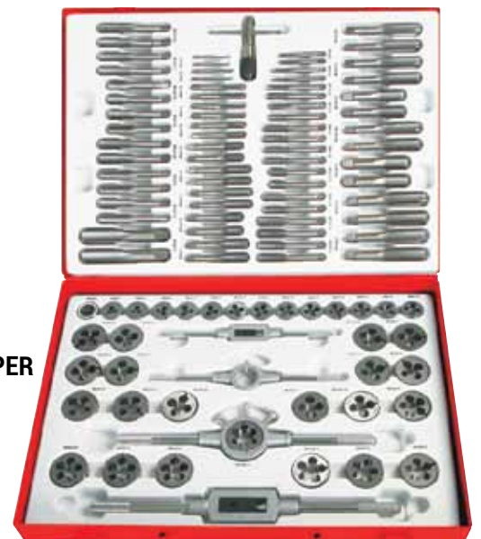
110 PCE METRIC, METRIC ISO & METRIC FINE • 1 each taper and intermediate taps • 1-tap wrench 1.6-11mm • 1-tap wrench 5-20mm • 1-die stock (1"/25.4mm OD) handle wrench • 1-die stock (1-1/2"/38.1mm OD) handle wrench • 1-'T' handle tap wrench • Metric: 2-18mm ISO & fine thread Part No. 748401100
